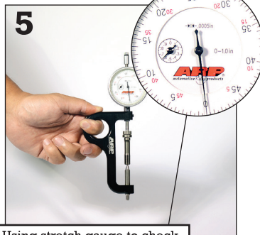
5 Using stretch gauge to check the original bolt length
