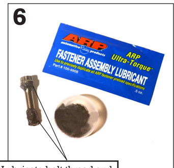
6 Lubricate bolt thread and under-head radius
