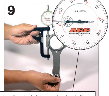
9 Using the stretch gauge to check the length of bolt again, make sure the stretch is correct. If not, tight or loose the bolt to correct the stretch
