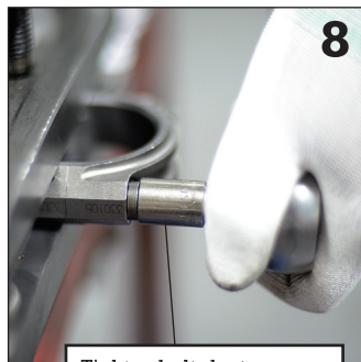
8 Tighten bolts by torque wrench in 2 times, refer to the recommended torque
